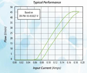
The above flow curve is a typical calibration record for the DVP. All proportional valves have a stored calibration data sheet readily available upon request.
