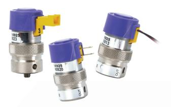
The EVP series proportional control valves combine the features of the existing EV series valve—long life, low power, and Clippard's reputation for high quality components— with the additional capability for proportional control. The EVP series valve provides air or gas flow control and varies the output flow based on the current input to the solenoid.
